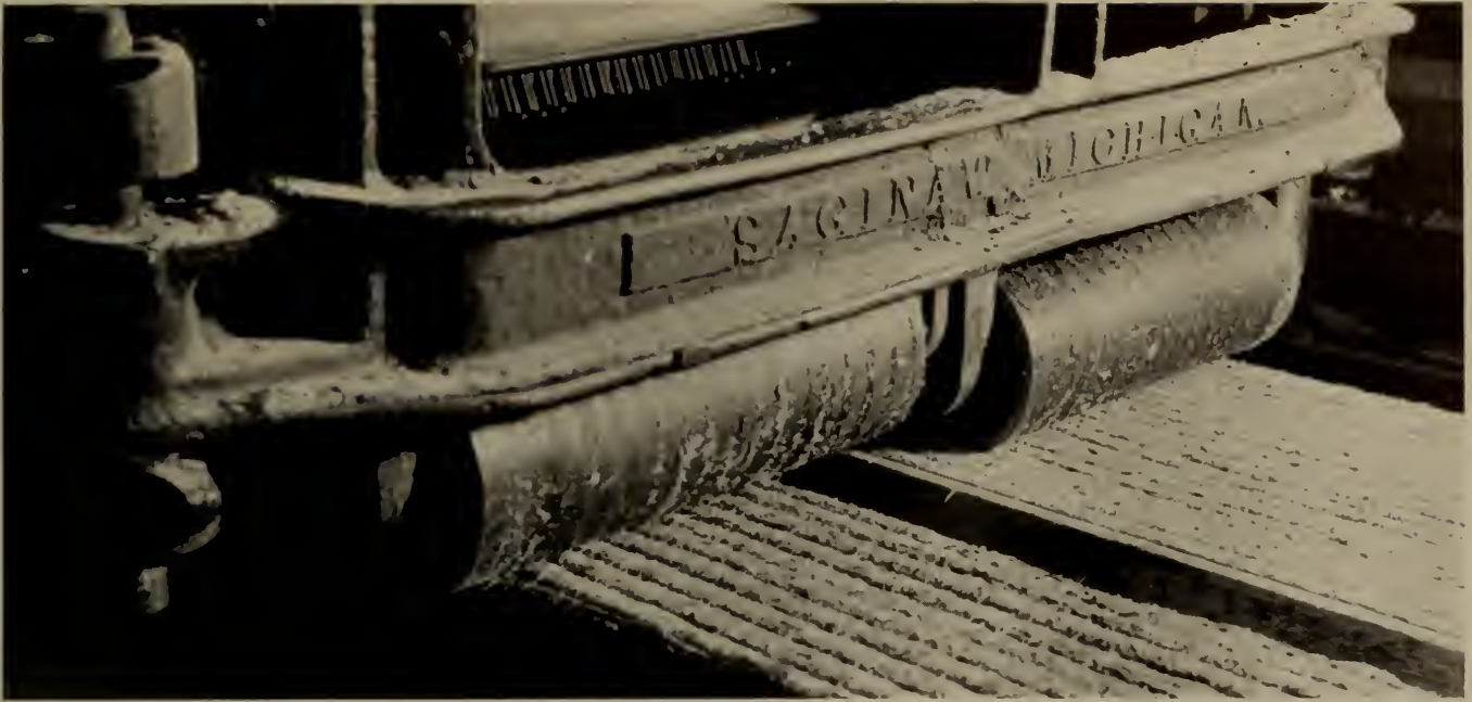
(Opposite) SAWYER'S-EYE-VIEW OF DOUBLE CUT BAND Saw is stopped for cameraman showing teeth on each edge of 14 inch width. Double-cuts require greater handling and sawing skill, more time in filing room, but speed up production since log is being sawed as carriage moves in each direction. (Photo courtesy West Coast Lumbermen's Association)
