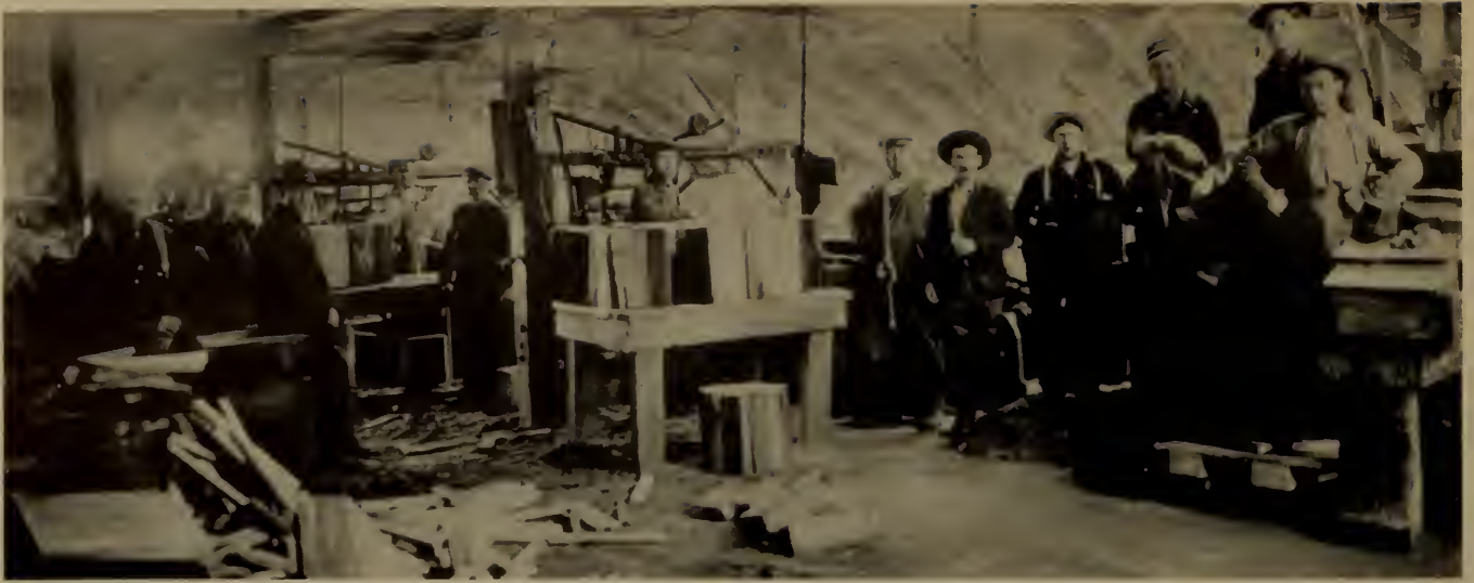
MILL AT DEMING, WASHINGTON — 1905 near McCleary. Shingle mills were usually on pond, river or lake for easiest transportation of logs and bolts. Also water kept wood clean and easier on saws. Brattle Brothers at Ridgefield taught shingle trade to many who set up own mills. Charles H. White was Brattle foreman for 24 years. (Photo courtesy C. H. White)
