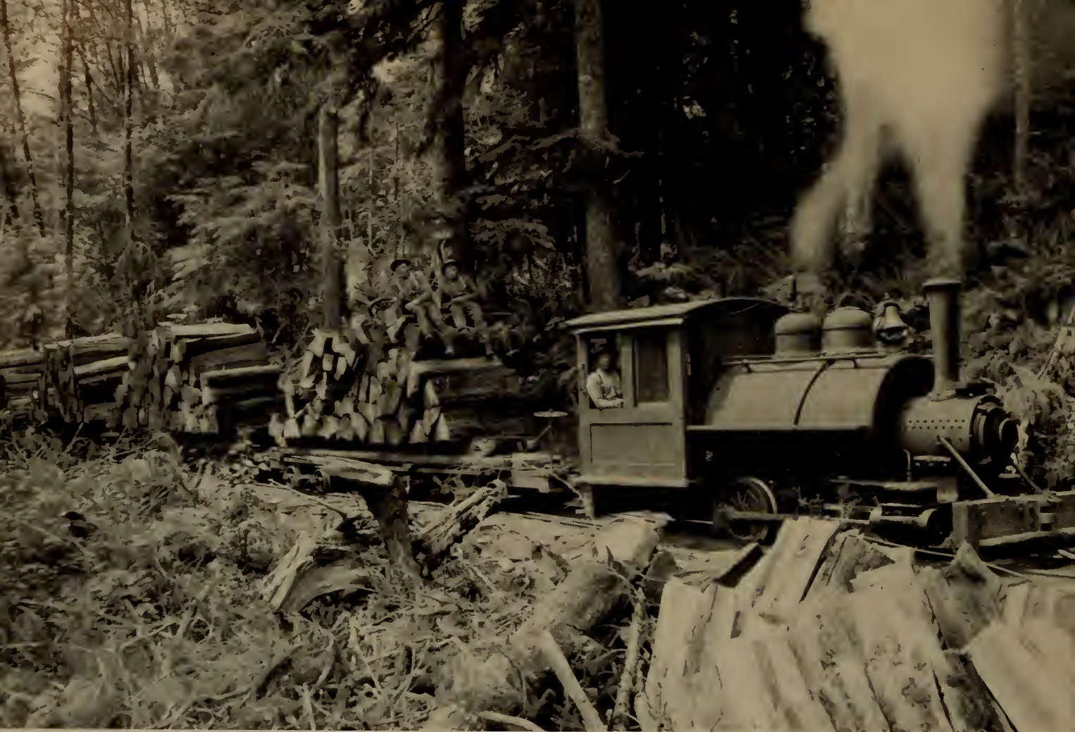
BOLT TRAIN Narrow gauge, saddle-tank lokey of Independent Coal and Coke Co. with sled loads of shingle bolts loaded on flat cars. (Darius Kinsey photo from Jesse E. Ebert Collection)
