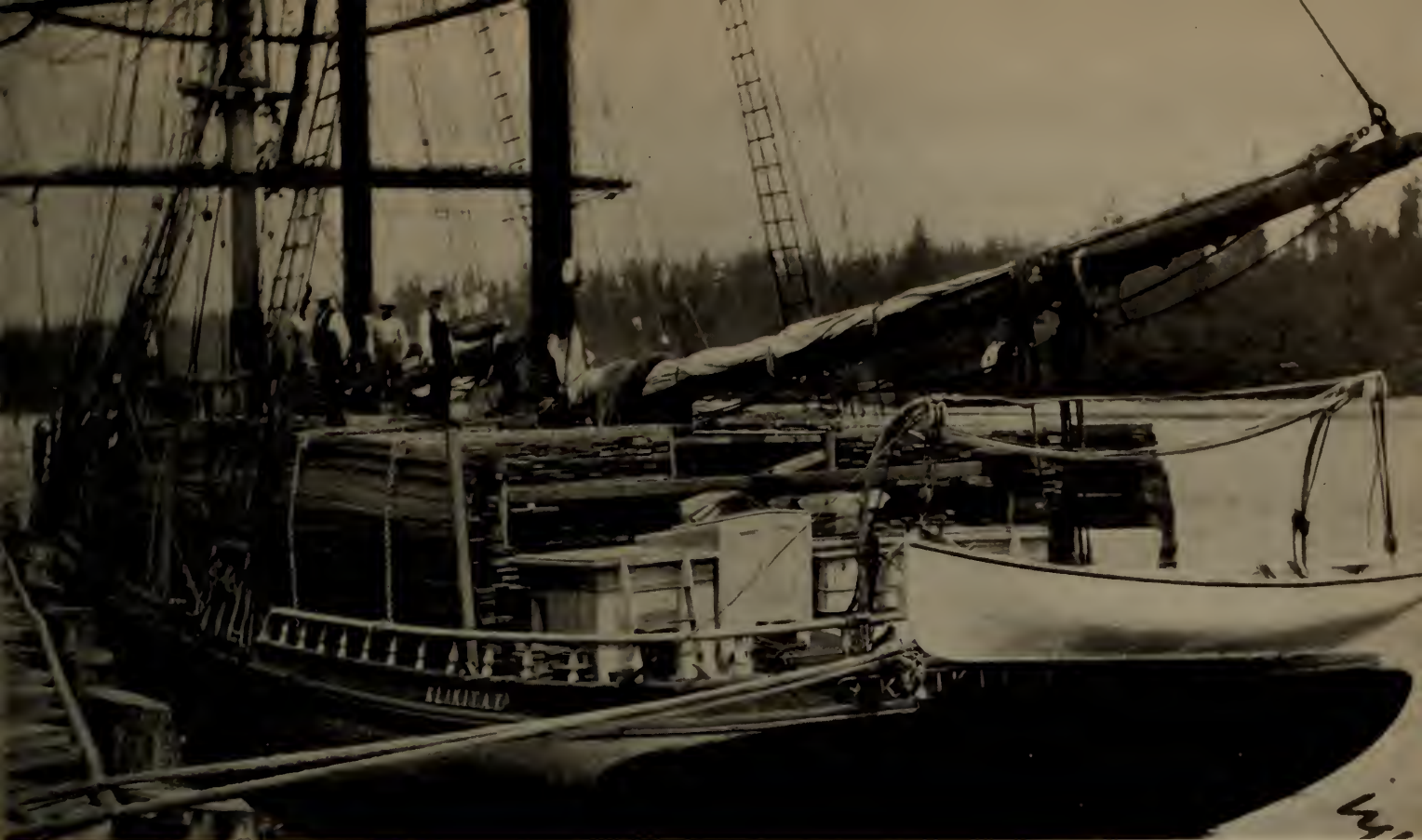
SCHOONER KLICKITAT was one of fleet on the regular run between Port Gamble, California and Hawaii. Twelve foot deck loads were customary cargo and more than often were swept overboard before ships cleared Cape Flattery. (Photo Ames Collection, University of Washington)
