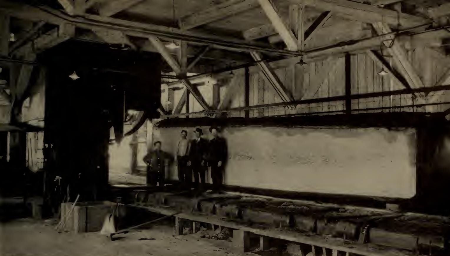
HEADSAW AND CARRIAGE AT SNOQUALMIE FALLS Lumber Co. a steady and important Weyerhaeuser producer and mainstay of economy in Snoqualmie Valley, Wash. Mill was built in 1916, managed by Warren, with Cutler Lewis as logging superintendent. (Darius Kinsey photo from Jesse E. Ebert Collection)
