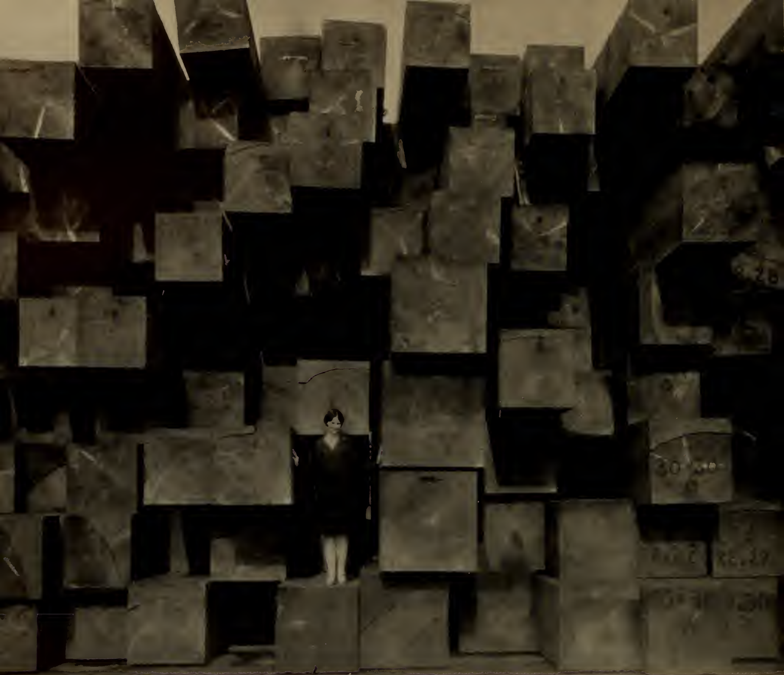
JAP SQUARES WERE STAPLE ITEM in '20s. 28"x28" and 30"x30" Douglas fir cants were standard export material to the Orient in the boom days of high mill production. (Photo courtesy West Coast Lumbermen's Association)
