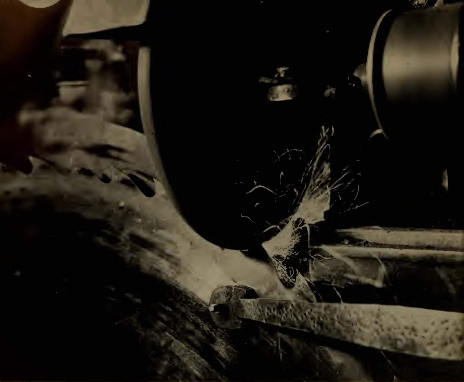
IN TO GET THEIR TEETH FIXED Automatic gumming and sharpening machine grinds gullets uniformly and buzzes shoulders and points of teeth in same operation. Number and size of saw teeth vary with type of lumber, speed of saw. (Photo courtesy West Coast Lumbermen's Association)
